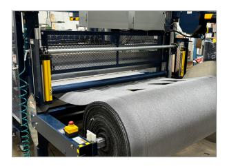
Our laminating capabilities offer our customers custom adhesive engineered solutions. Materials can be laminated together to provide sound, moisture, contamination, and thermal barriers.
