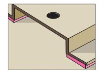
3M<sup>™</sup> VHB<sup>™</sup> Tapes bond panel stiffeners, on contact, to pre-painted metal cabinetry. Unlike welding, applying the tape does not damage the finish.
