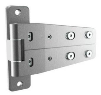
**CHOOSING THE RIGHT HINGE FOR HVAC UNITS:** This zinc die-cast and plated 3-axis adjustable hinge for insulated doors (P/N 321158) by Allegis Corporation provides a 180-degree opening. Because it can be adjusted for X, Y and Z axis, it offers the flexibility that mechanical engineers designing HVAC systems need to reduce leakage while maintaining ease-of-maintenance for service techs.
